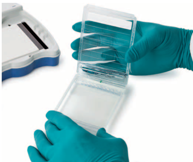
Fig 2D. The edge of the upper section of the cassette is used to remove excess gel in preparation for downstream processing.
