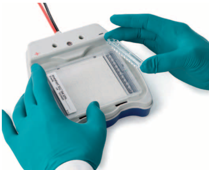
Fig 2A. Amersham ECL Gel comes securely enclosed in a plastic cassette. The entire cassette is placed in the Amersham ECL Gel Box. The comb is removed to expose the wells for sample loading.
