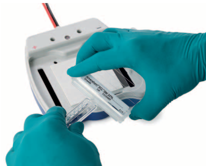
Fig 2C. No additional tools are needed; the comb is used as a tool to open the cassette.
